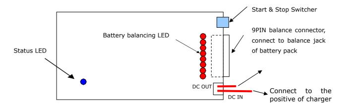
There is 1 balance socket and 2 leads on the right of CY – B8+. You should assure the connection in accordance with CONNECTION DIAGRAM.
