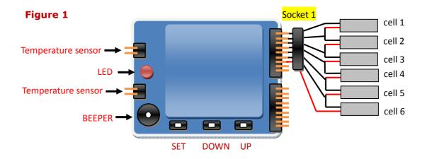
2. For two battery packs, connect them in series first and then plug battery 1# into socket 1, and battery 2# into socket 2 separately. Take one 8S battery and one 4S sample as following:
