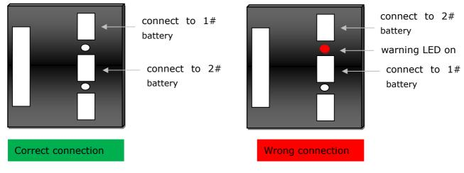
Connect adapter wire to charger balance port, then connect total battery pack positive to charger output port B+, and finally connect battery negative to output port B-
